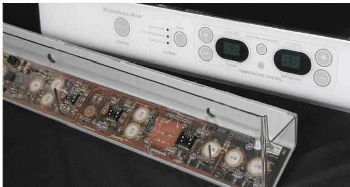
*TouchSensor provided Whirlpool a custom solution by working with the OEM's preferred supplier. The end result is a glass-like, injection-molded control panel both for the main user interface (shown) and controls for two independent deli trays.*
