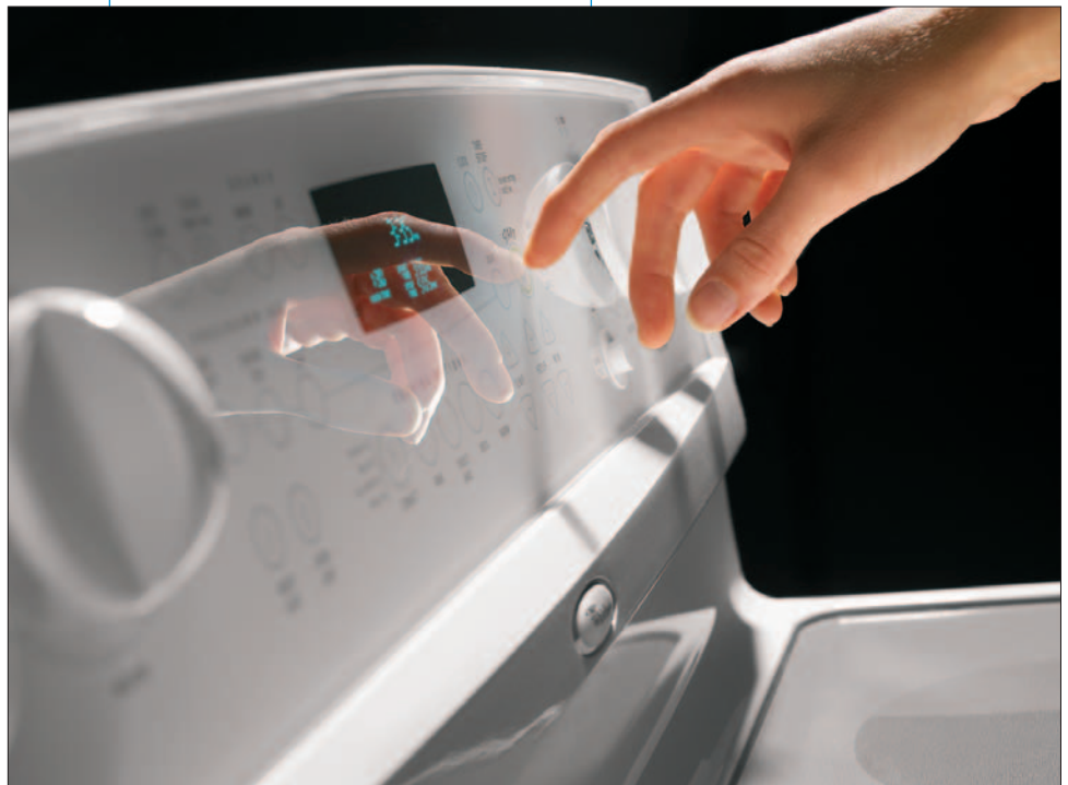
Glass touch control panels are featured in a line of Whirlpool freestanding electric ranges, built in Tulsa, OK, U.S. The panels use field-effect switches that sense a conductive mass, such as a finger, through the glass.
